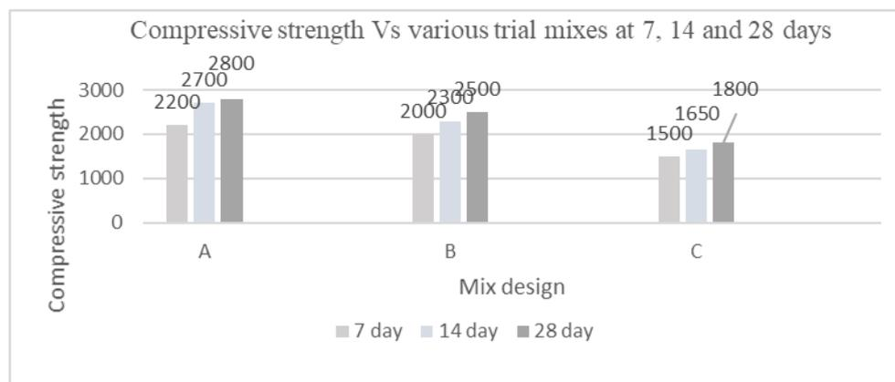
Figure 4: Compressive Strength of various sand cement block mixes with SP-1 at 7, 14, and 28 days.
