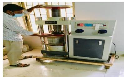
i) Sand Cement Solid Block tested by UTM Machine
