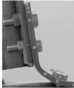
(c) Deformation of top angle after test (Hasan et al., 2019)
