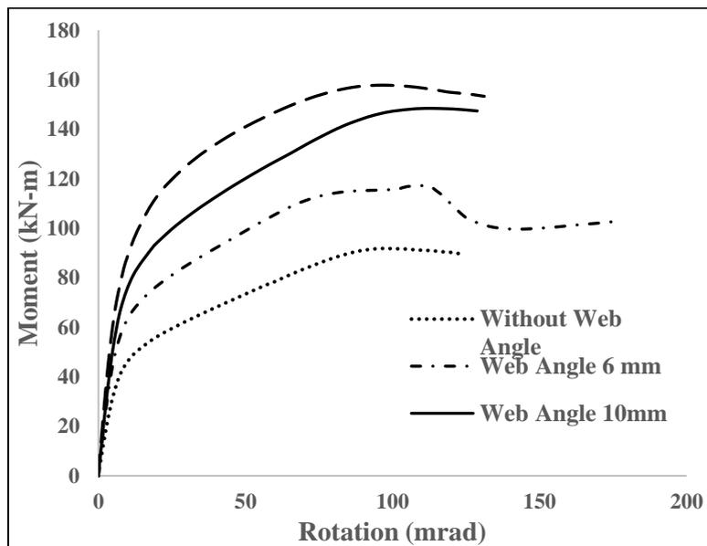
Figure 9: Moment vs Rotation Curve for Web Angle thickness analysis
