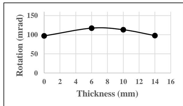
Figure 11: Rotation-Thickness curve for Web angle thickness analysis
