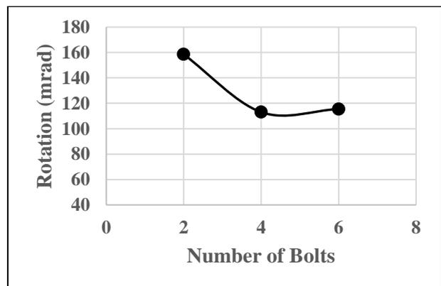
Figure 15: Rotation vs Number of Seat Bolts in Beam curve
