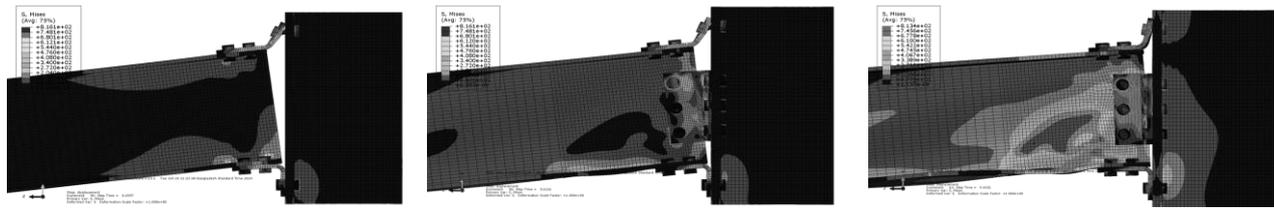
(a) Without Web-angle      (b) Web angle thickness 6 mm      (c) Web angle thickness 14 mm
