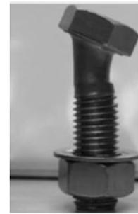
(e) Deformation of bolt after test (Hasan et al., 2019)
