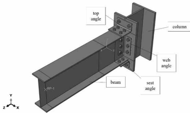
Figure 1: Details of joint
