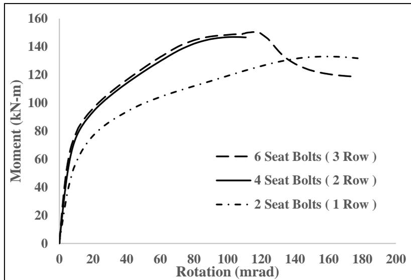
Figure 13: Moment vs Rotation Curve for Top-Seat Bolts in Beam Flange Analysis
