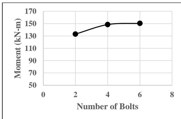
Figure 14: Moment vs Number of Seat Bolts in Beam curve
