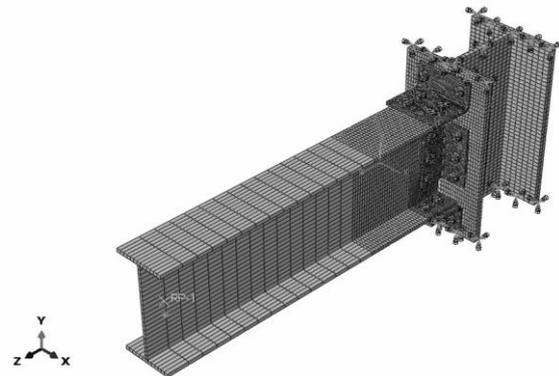
Figure 2: Loading and support condition on the meshed model
