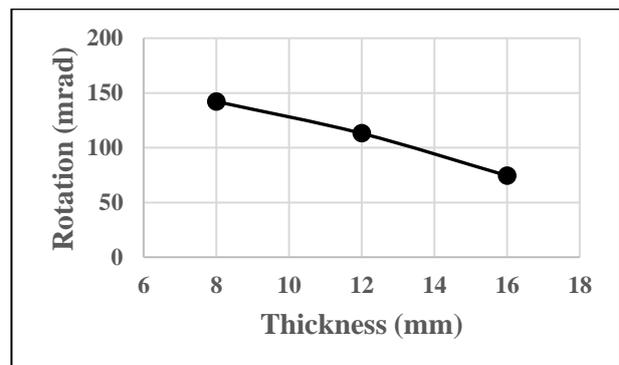
Figure 7: Rotation-Thickness curve for top-seat angle thickness analysis
