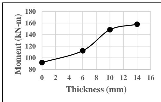
Figure 10: Moment-Thickness curve for Web angle thickness analysis
