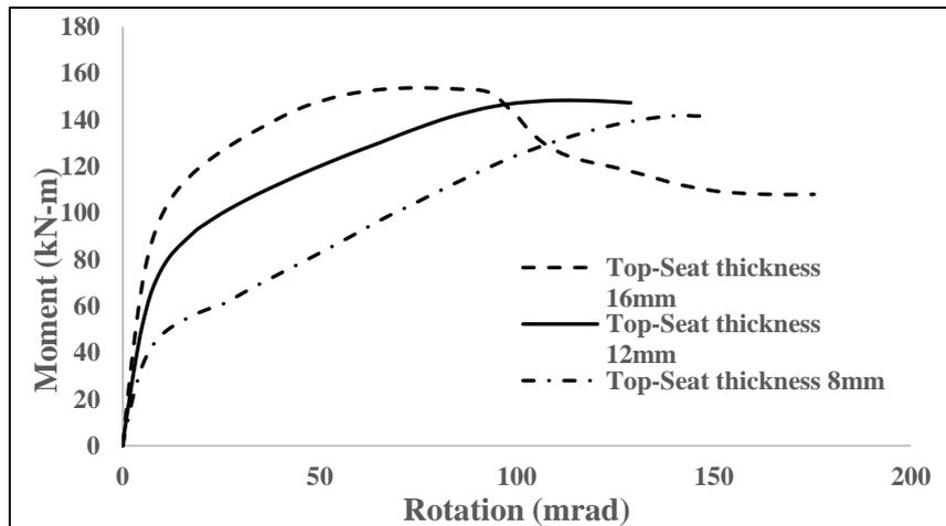
Figure 5: Moment-Rotation curve for top-seat angle thickness analysis
