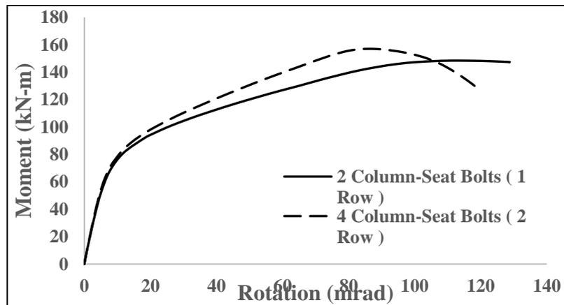
Figure 17: Moment vs Rotation Curve for Top-Seat Bolts in Column Flange Analysis
