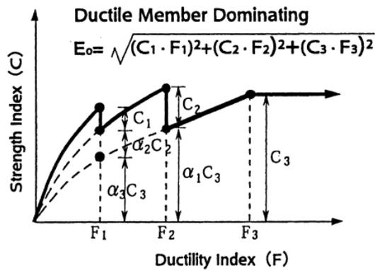
**Figure 2:** Basic seismic index of ductility-dominant structure (Fukuyama et al., 2000)
