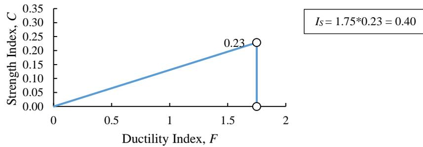
**Figure 6:** Seismic capacity along Y-direction (short direction).
