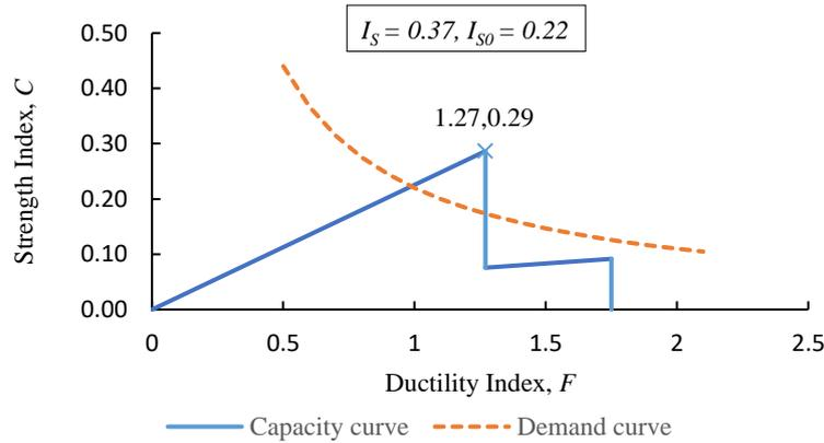
**Figure 7:** Demand and capacity comparison for X-direction (long direction).
