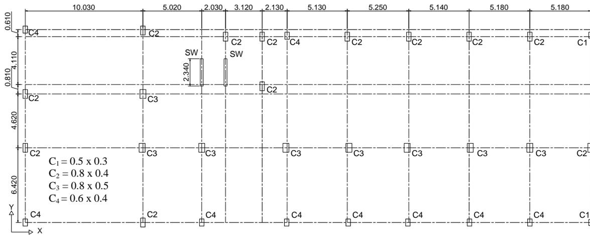
**Figure 4:** Column layout of the building (all dimensions are in meter).
