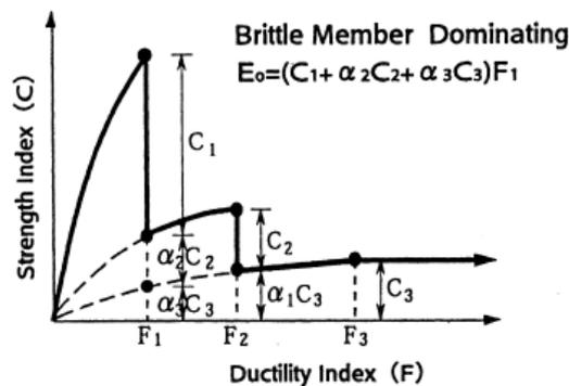
**Figure 3:** Basic seismic index of strength-dominant structure (Fukuyama et al., 2000)
