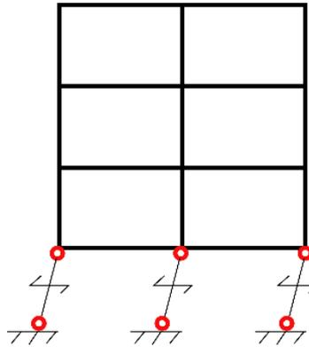
**Figure 1:** Story collapse mechanism. (JBDPA 2016)
