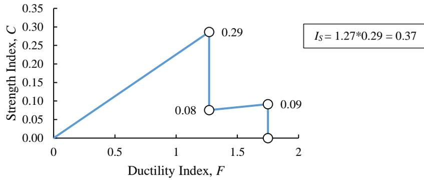
**Figure 5:** Seismic capacity along X-direction (long direction).
