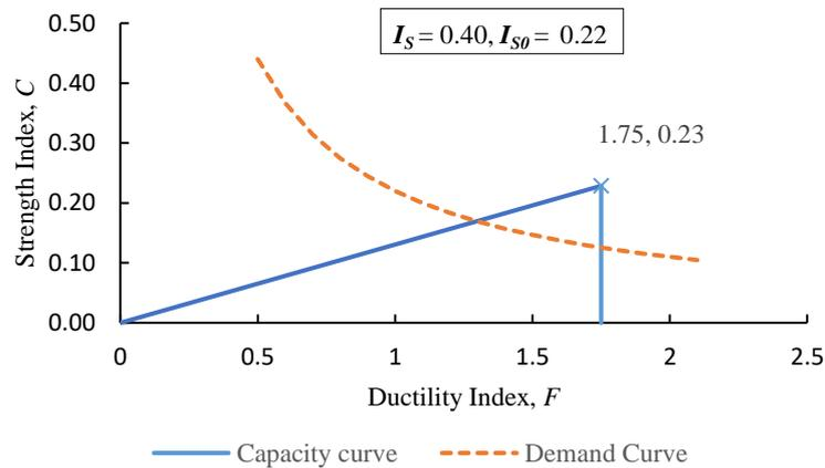
**Figure 8:** Demand and capacity comparison for Y-direction (short direction).
