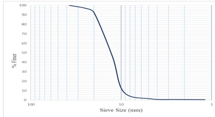
Figure 1: Grain size distribution curve of recycled aggregate
