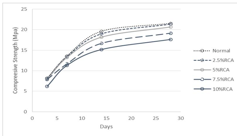
Figure 5: Comparison of Compressive Strength of RCA
