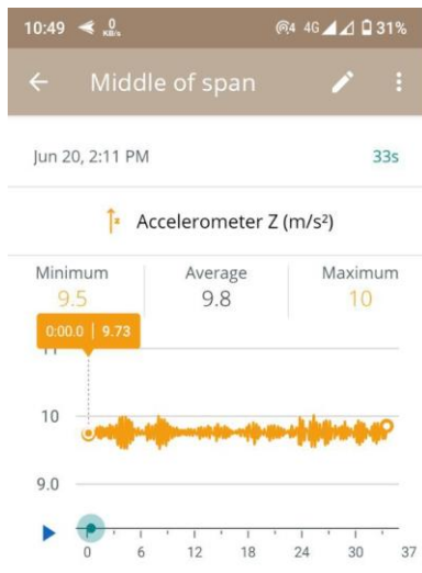
Figure 5: Midspan raw accelerometer data collection at Mohonpur Bridge
