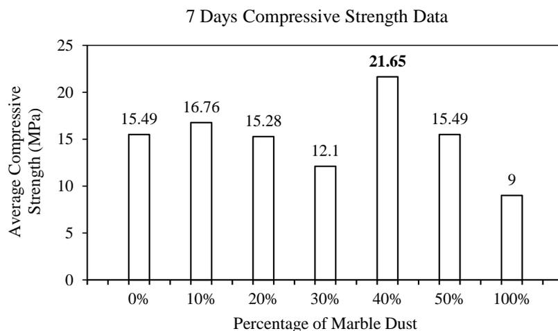
Figure 4 : Bar diagram showing the variation in strength for 7 days test
