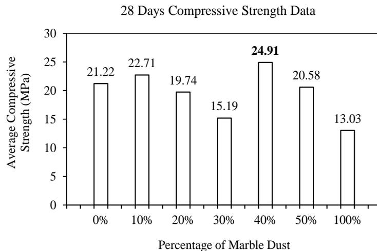
Figure 6 : Bar diagram showing the variation in strength for 28 days test
