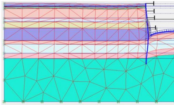
Figure 1: Numerical model of WJD-11 section (Deformed shape)
