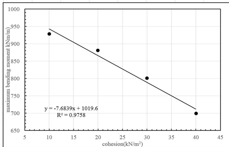
Figure 6 Relation between cohesion and maximum bending moment of diaphragm wall
