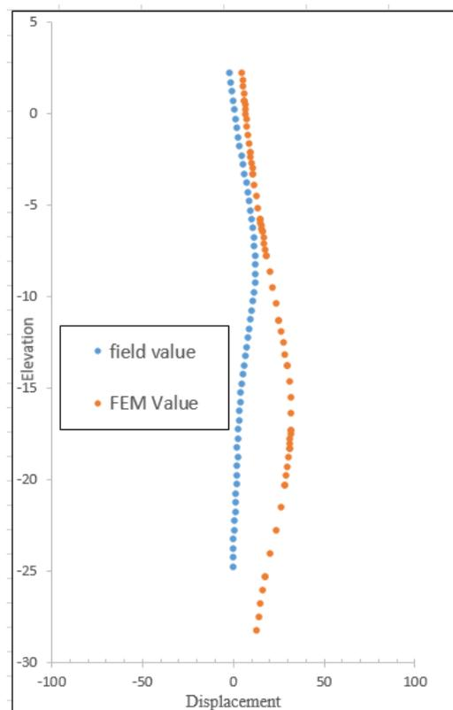
Figure 2: Comparison between field and predicted value at WJD-11 section
