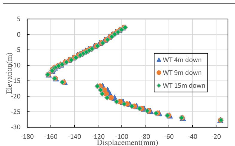
Figure 4 Relation between Max displacement and depth of water table of the soil profile
