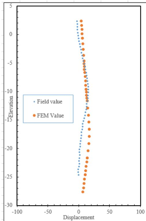
Figure 3: Comparison between field and predicted value at EJD-02 section
