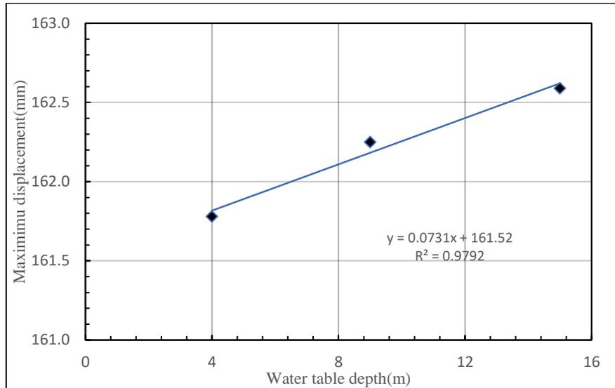
Figure 5 Relation between maximum displacement and depth of water table of the soil profile
