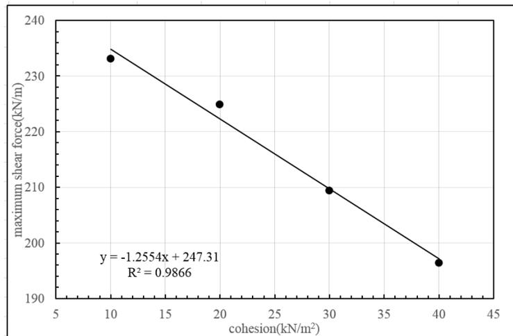
Figure 7 Relation between cohesion and maximum shear force of diaphragm wall
