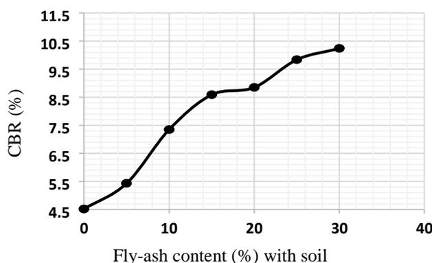
Figure 7 Variation of CBR vs. mixing percentage of fly-ash
