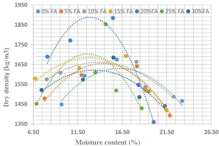
Figure 4: Variation of moisture content with dry density for fly-ash
