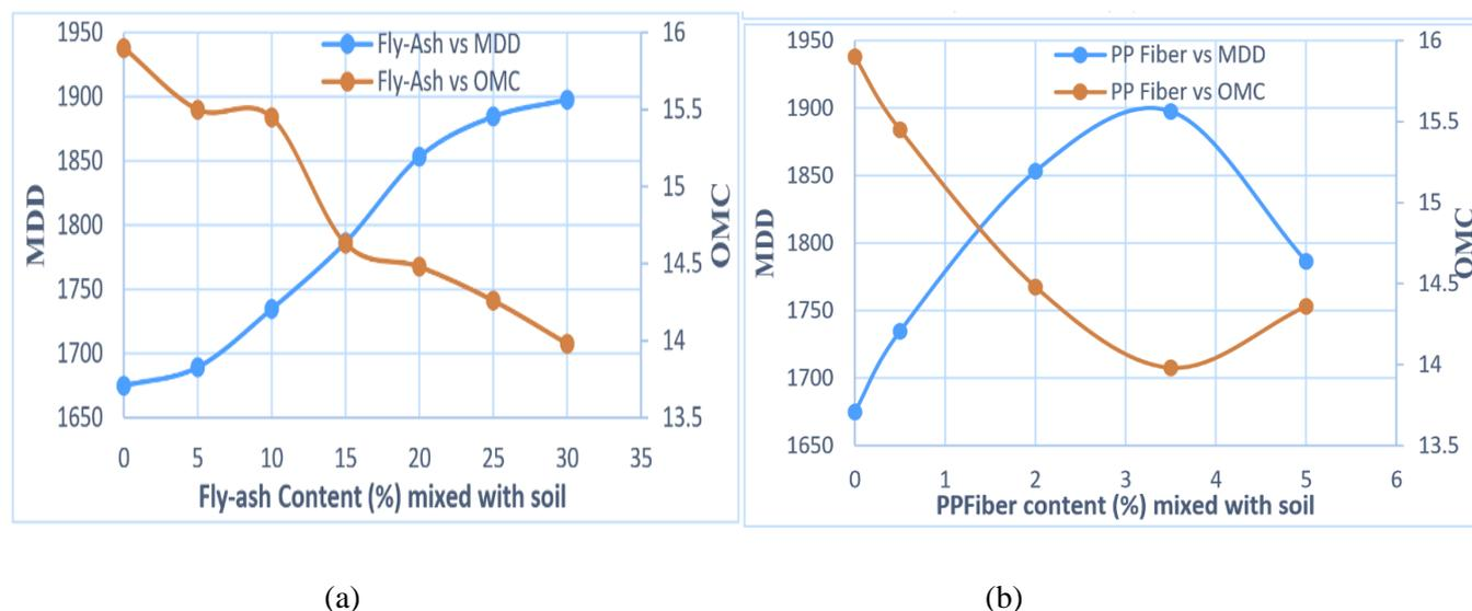
Figure 6: Variation MDD and OMC of stabilized soils (a) fly-ash (b) polypropylene fibre
