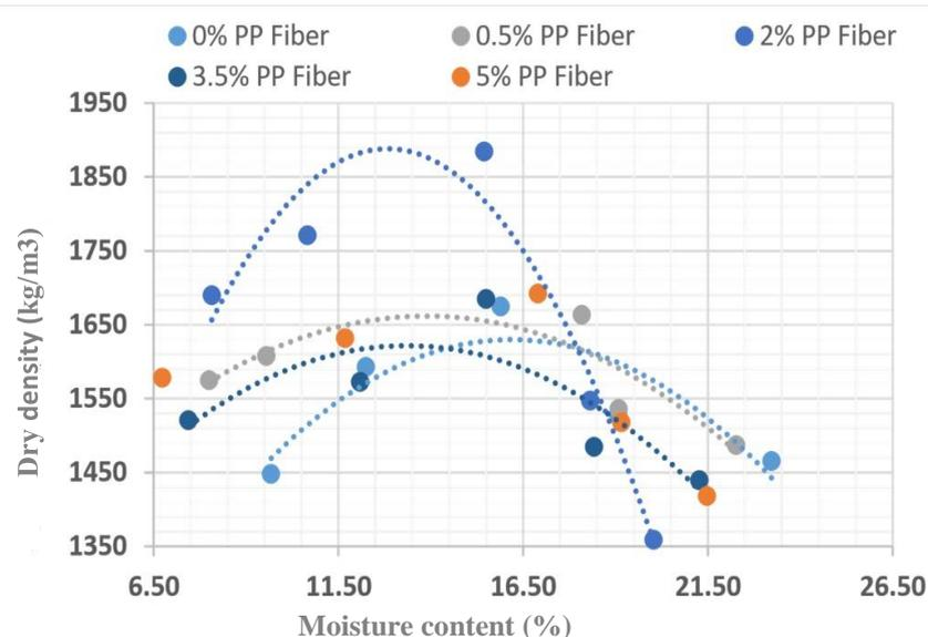
Figure 5: Variation of moisture content with dry density for Polypropylene Fibre
