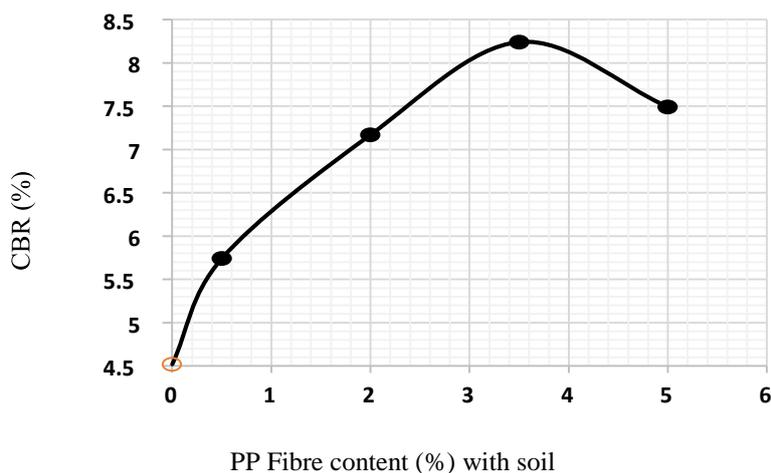
Figure 8: Variation of CBR vs. mixing percentage of polypropylene fibre
