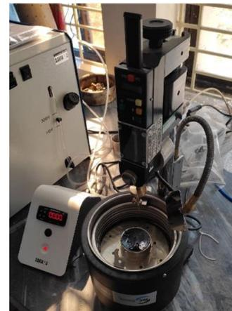
Figure 2: Penetration Test Apparatus
