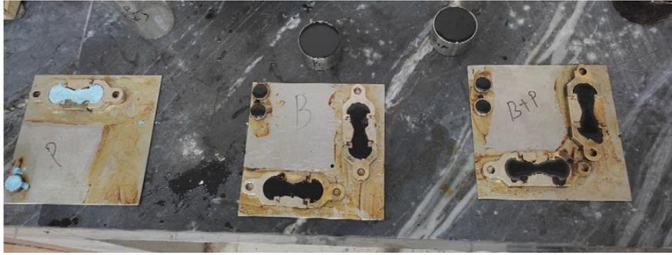
Figure 1: Bitumen, Polypropylene and Bitumen and Polypropylene Mix Sample preparation
