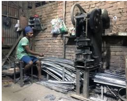
Figure 5: The cutting process of old ship's plate for making the angle and railing(Captured by Author, October,2021)
