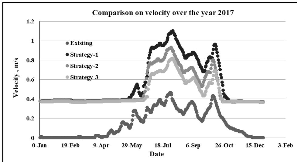
Figure 7: Velocity profile before and after dredging
