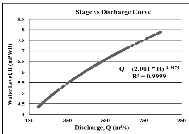
Figure 6: Rating curve using conveyance analysis
