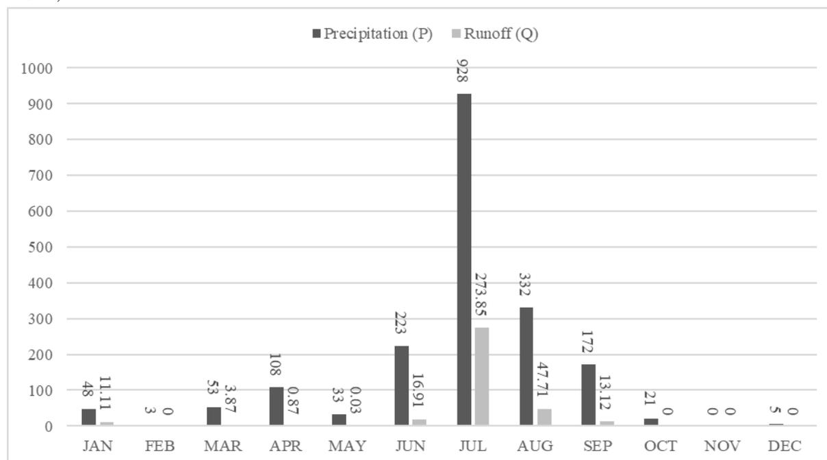
Figure 10: Surface runoff with respect to precipitation.
