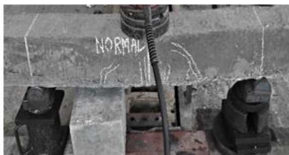
(a) Cracks in normal RCC beam
