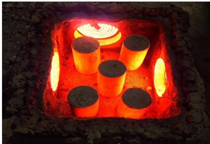
Figure 3: Burning of the specimens
