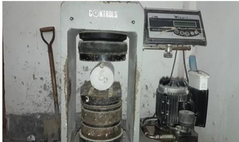
Figure 6: Typical setup for splitting tensile strength determination
