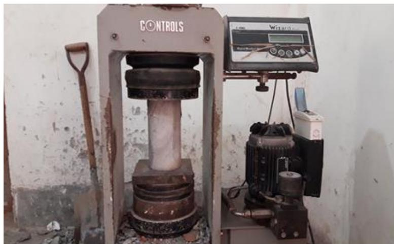
Figure 5: Typical test set-up for determination of crushing strength of concrete
