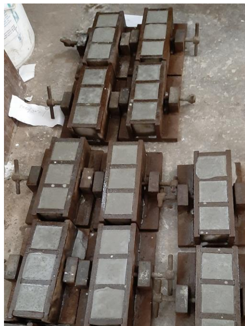
Figure 2: Casting of grout samples
