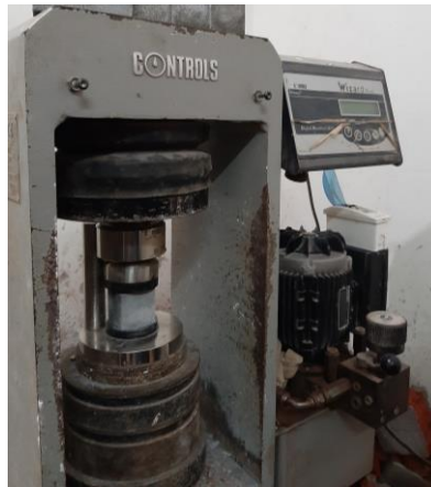
Figure 3: Placement of the cube in the testing machine
