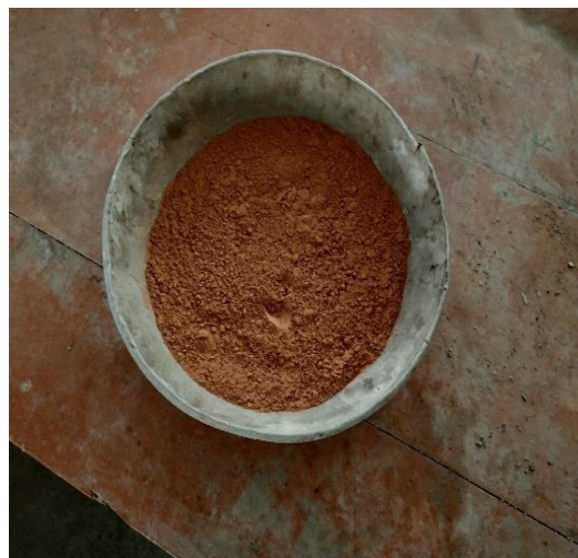
Fig 2: Preparation of ceramic waste powder through #200 passing
