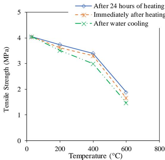
Figure 6: Tensile strength at different elevated temperatures
