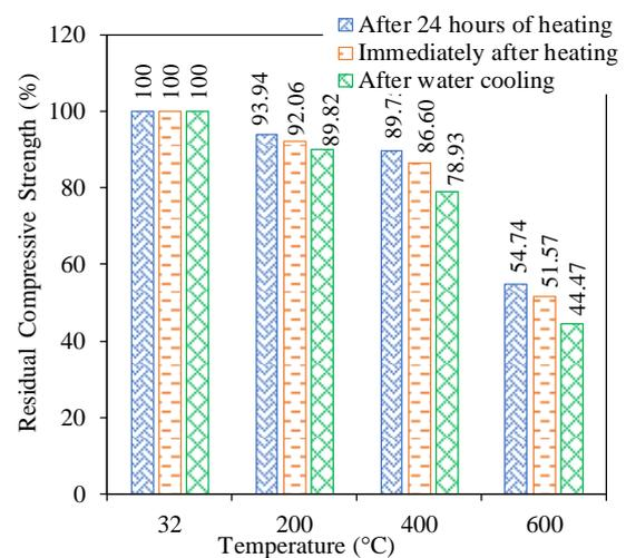
Figure 5: Residual compressive strength at different elevated temperatures
