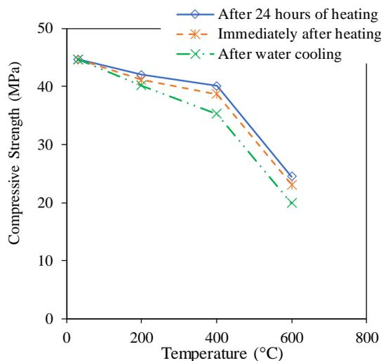
Figure 4: Compressive strength at different elevated temperatures
