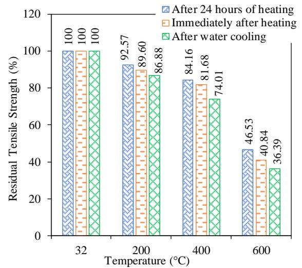
Figure 7: Residual tensile strength at different elevated temperatures
