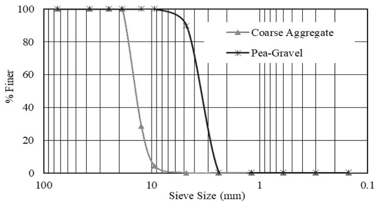
Figure 6: Gradation Curve for Coarse Aggregate and Pea-Gravel
