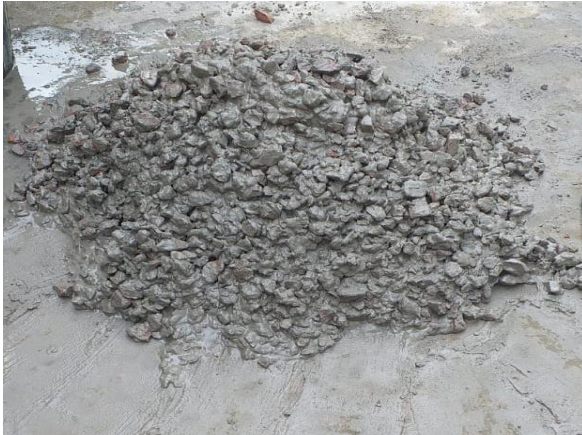
Fig. 3: Concrete mixture (M20)
