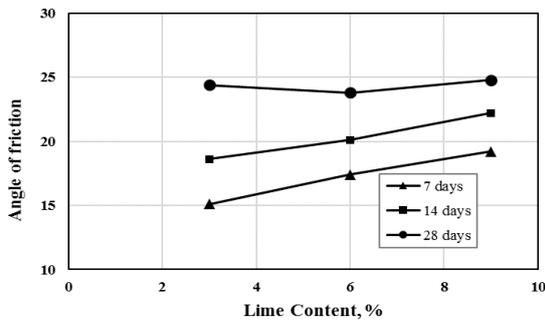
Figure 20: Effect of Lime Content on Effective Angle of Friction
