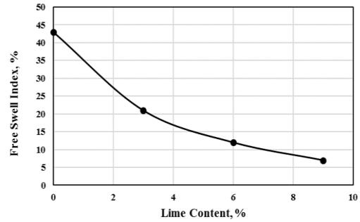
Figure 9: Effect of Lime on Free Swell Index
