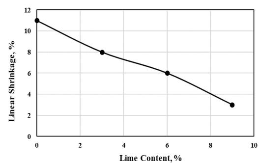
Figure 7: Effect of Lime on Linear Shrinkage
