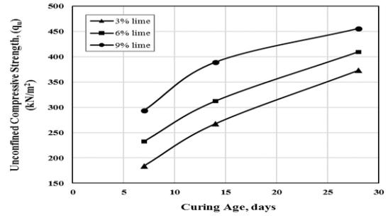
Figure 15: Effect of Curing Age on Unconfined Compression Strength
