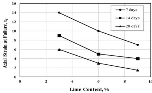
Figure 16: Effect of Lime Content on Axial Strain at Failure
