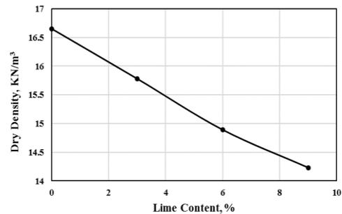
Figure 13: Effect of Lime on Maximum Dry Density
