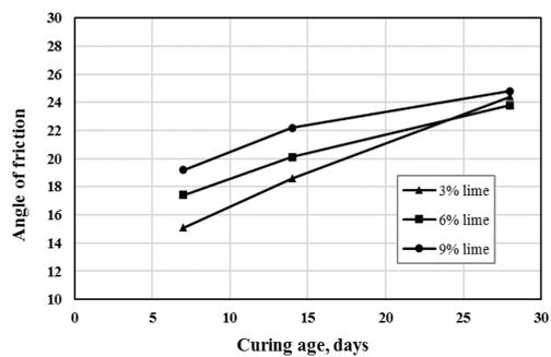
Figure 21: Effect of Curing Age on Effective Angle of Friction
