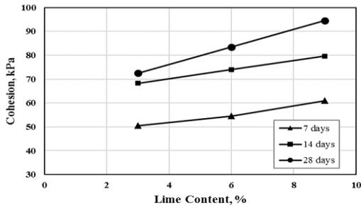
Figure 18: Effect of Lime Content on Effective Cohesion
