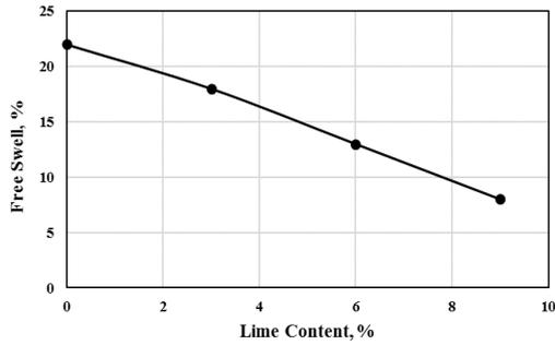
Figure 8: Effect of Lime on Free Swell
