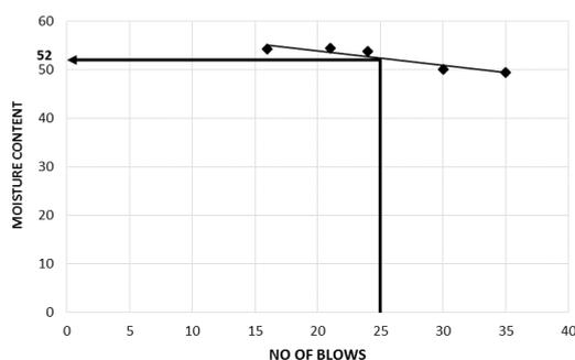
Figure 1: Flow Curve
