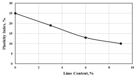
Figure 6: Effect of Lime on Plasticity Index
