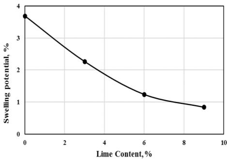
Figure 10: Effect of Lime on Swelling Potential
