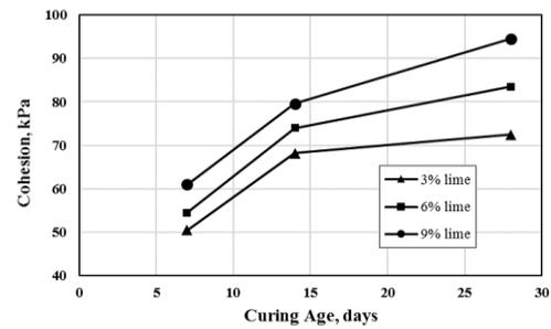
Figure 19: Effect of Curing Age on Effective Cohesion
