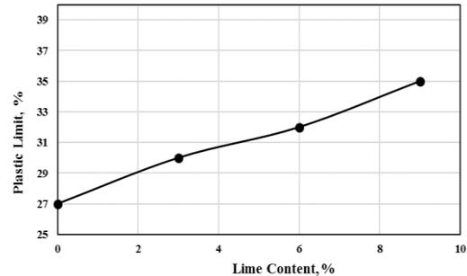
Figure 5: Effect of Lime on Plastic Limit
