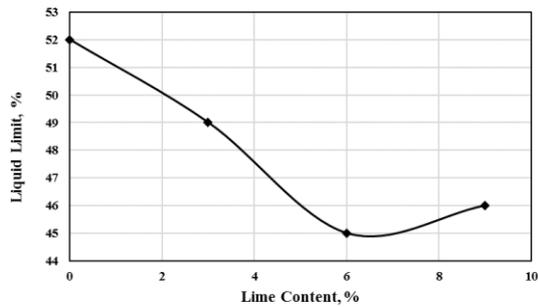
Figure 4: Effect of Lime on Liquid Limit
