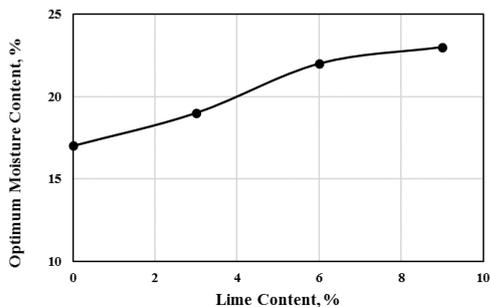
Figure 12: Effect of Lime on Optimum Moisture Content
