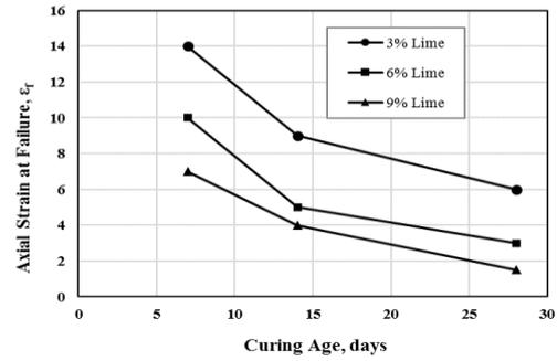
Figure 17: Effect of Curing Age on Axial Strain at Failure
