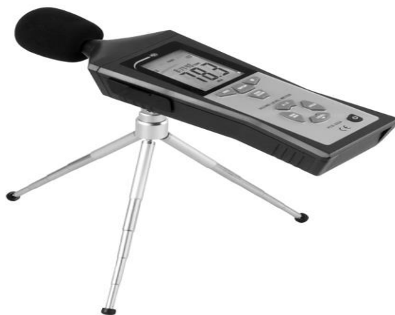
Figure 3: Noise Data sampling by Sound Level Meter
