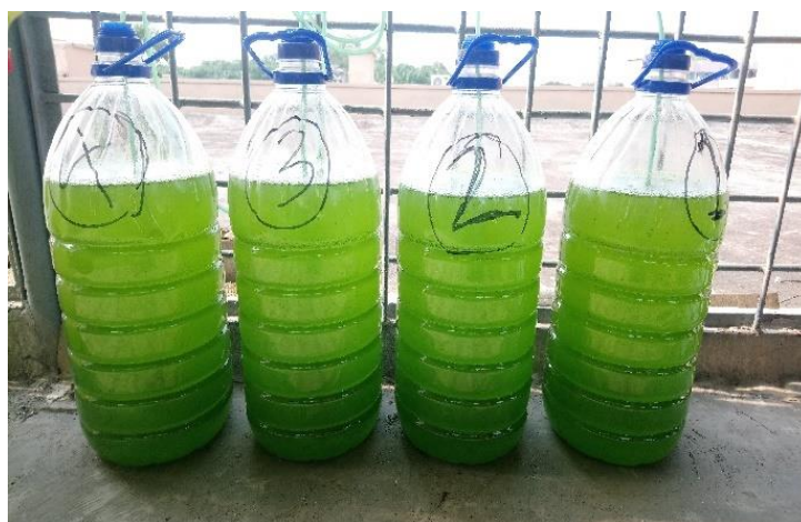
Figure 2 (a): Microalgae cultivation in photobioreactor (PBR)
