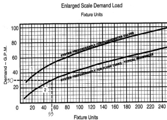
Figure 3.5: Fixture Unit vs Demand (gpm) Graph
