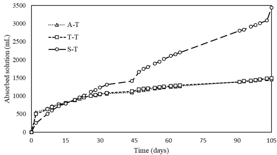
Figure 3: Cumulative absorption of tap water with time
