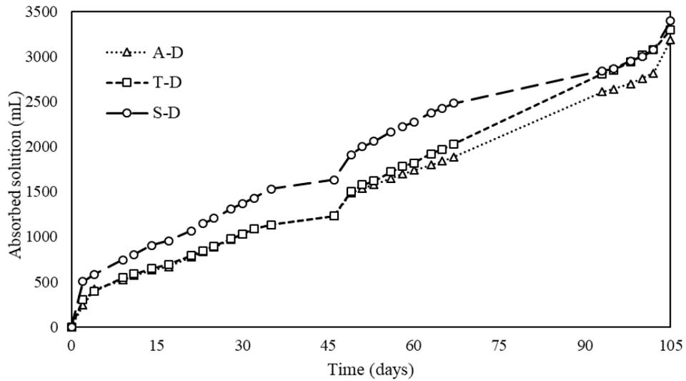
Figure 2: Cumulative absorption of distilled water with time
