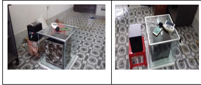
Figure 2: Acoustic properties test of Composite panels
