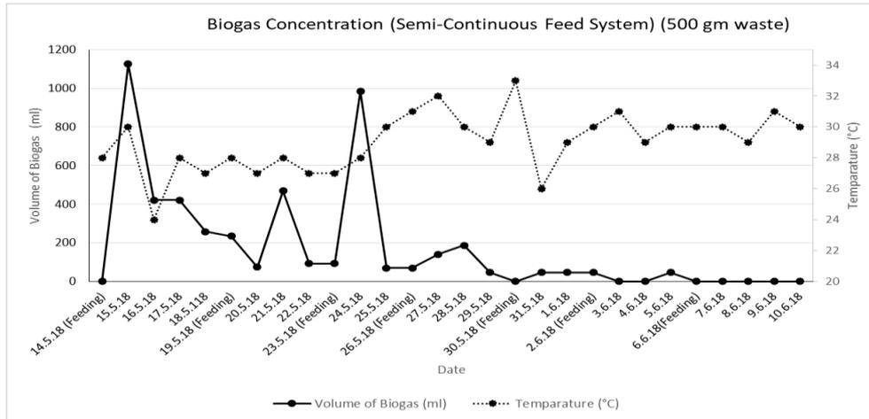
Figure 3.4: Bio-gas(black line) and temperature variation (ash line) for 500gm of waste
