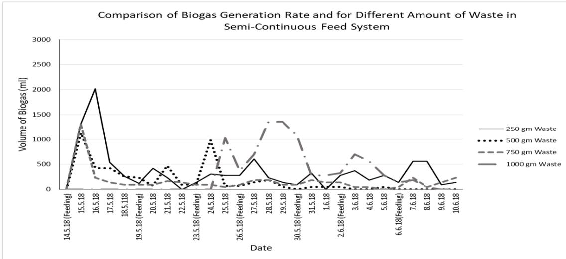
Figure 3.7: Bio-gas generation comparison from 3<sup>rd</sup> experiment
