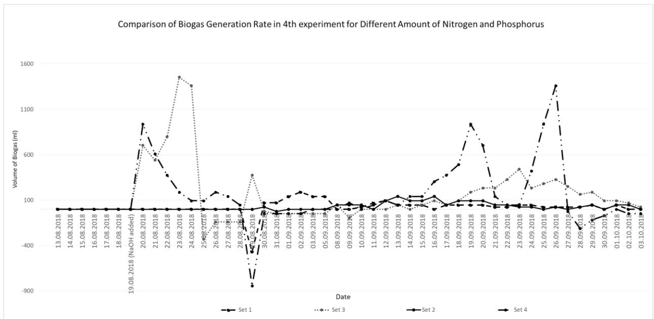
Figure 3.12: Bio-gas generation comparison from 4<sup>th</sup> experiment
