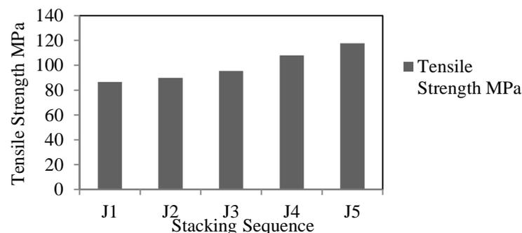
Figure 1: Variation of tensile strength with stacking sequence
