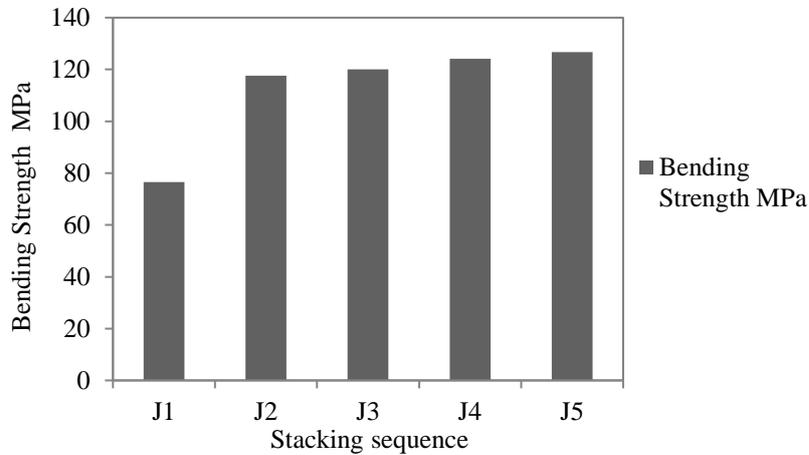
Figure 2: Variation of Bending strength (BS) with stacking sequence
