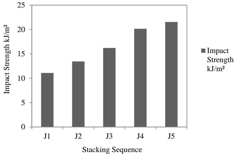
Figure 4: Impact strength with increasing stacking sequence
