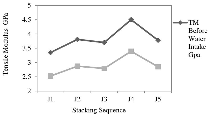
Figure 8: Reduction of Tensile Modulus for Soil degradation
