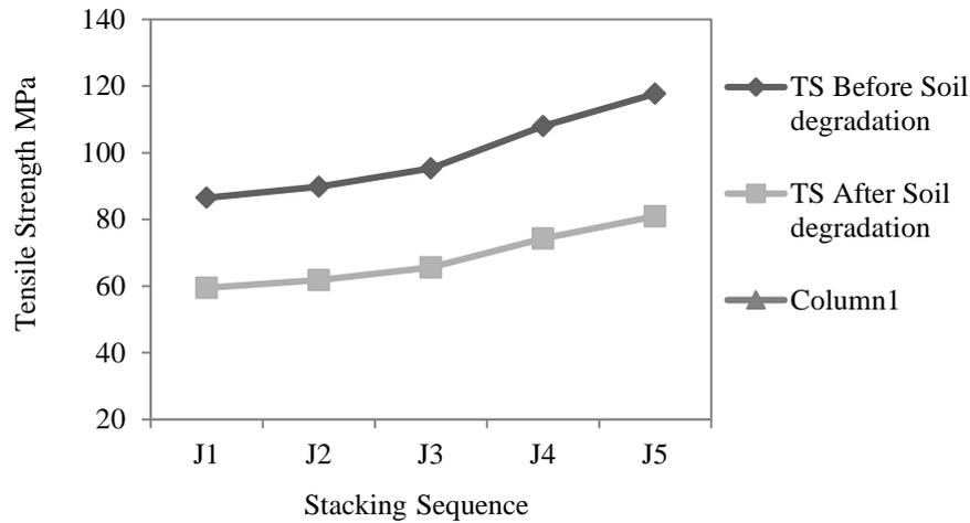
Figure 6: Reduction of tensile properties for Soil degradation
