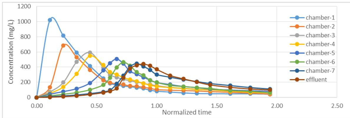
Figure 5. RTD results of various chambers.
