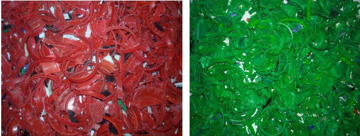
Figure Error! No text of specified style in document.. Filter media used in the study.
