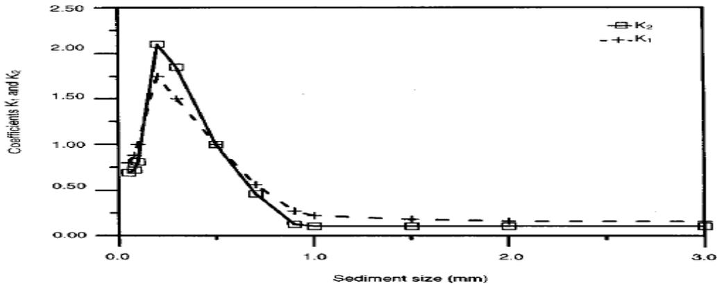
Figure 1: Coefficients  $K_1$  and  $K_2$  versus sediment size (Abdulaziz A. A. and Matin M.A., "Fluvial Stage-discharge Rating of Wadi Hanifa Main Channel", Journal of King Saud University, Engineering Sciences: 12(1); 45-63.)
