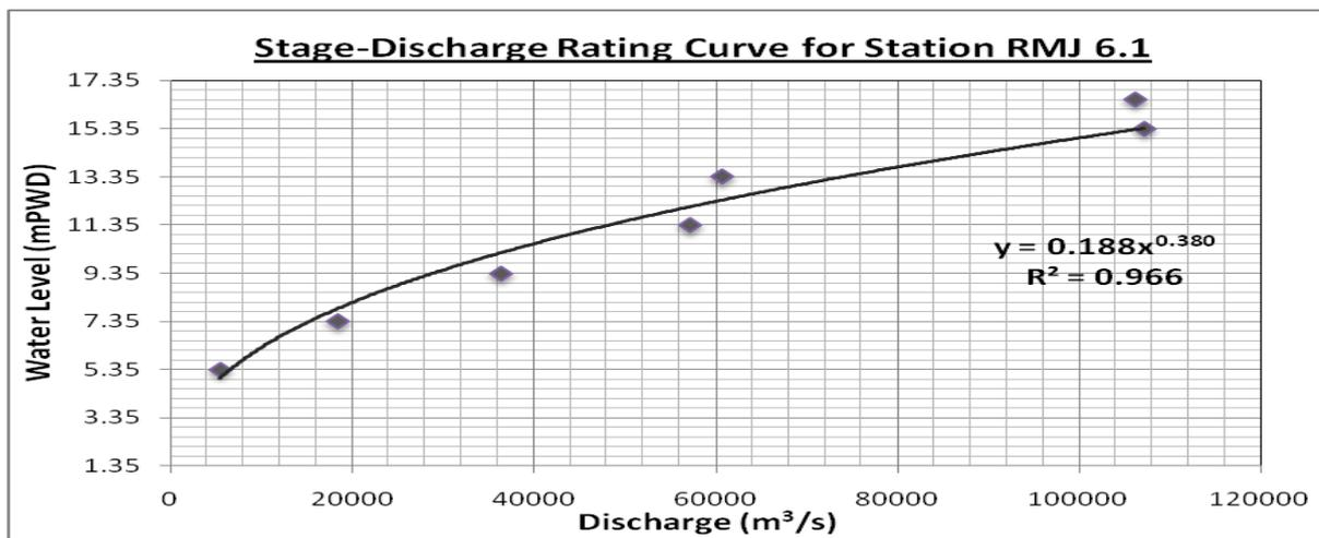
Figure 4: Typical stage-discharge rating curve for station RMJ 6.1.
