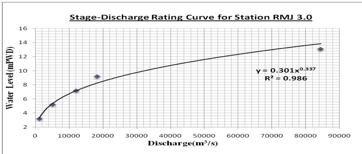
Figure 5: Typical stage-discharge rating curve for station RMJ 3.0
