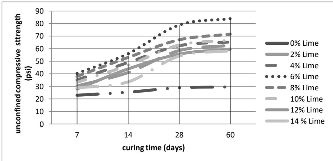
Figure 4: Unconfined compressive strength of Hilly soil as a function of curing period for eight different lime soil mixtures
