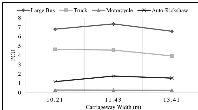
Figure 2: The Effect of Carriageway Width on PCU for Motorized Vehicles
