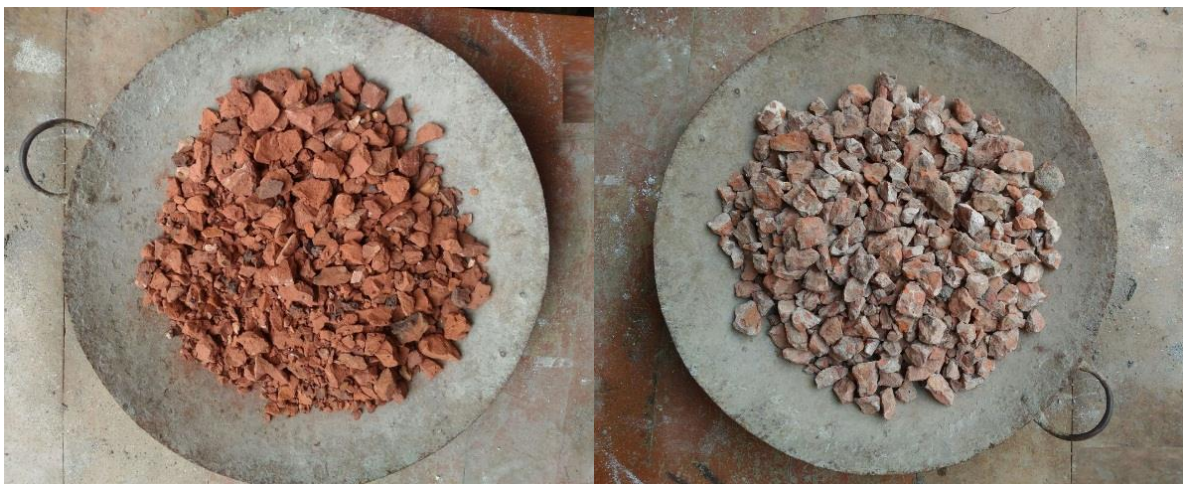
Figure 2: Natural Aggregate & Recycled Aggregate
