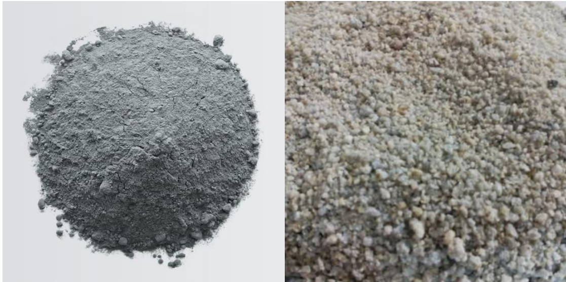
Figure 3: Fly Ash and Blast Furnace Slag
