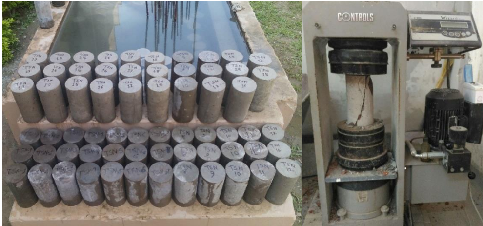
Figure 4: Illustration of prepared sample for compressive strength test
