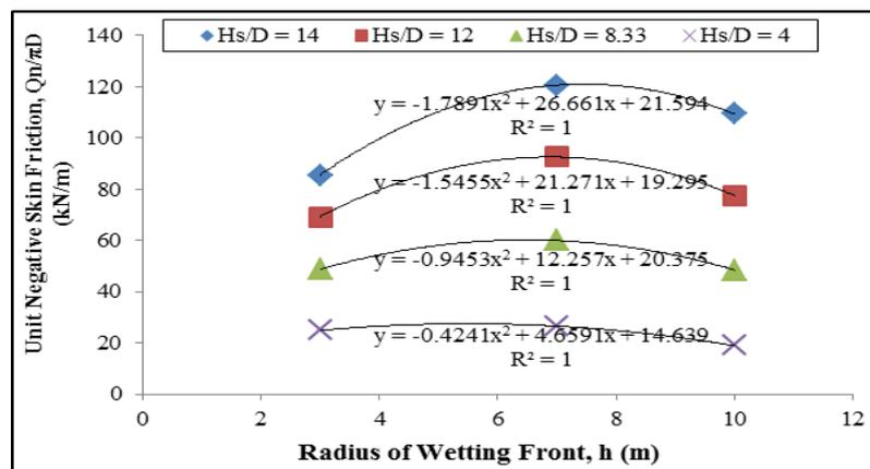
Figure 10: Effect of radius of wetting front (h) on  $(Q_n/\pi D)$ , when  $C_p = 10\%$ .
