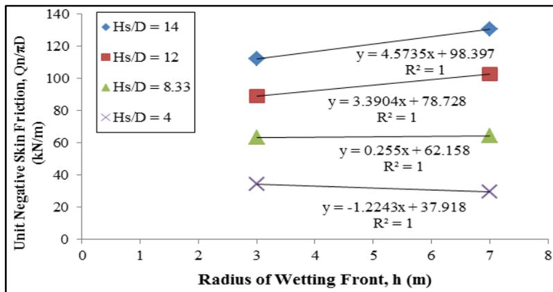
Figure 11: Effect of radius of wetting front (h) on  $(Q_n/\pi D)$ , when  $C_p = 15\%$ .
