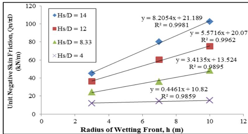
Figure 9: Effect of radius of wetting front (h) on  $(Q_n/\pi D)$ , when  $C_p = 5\%$ .
