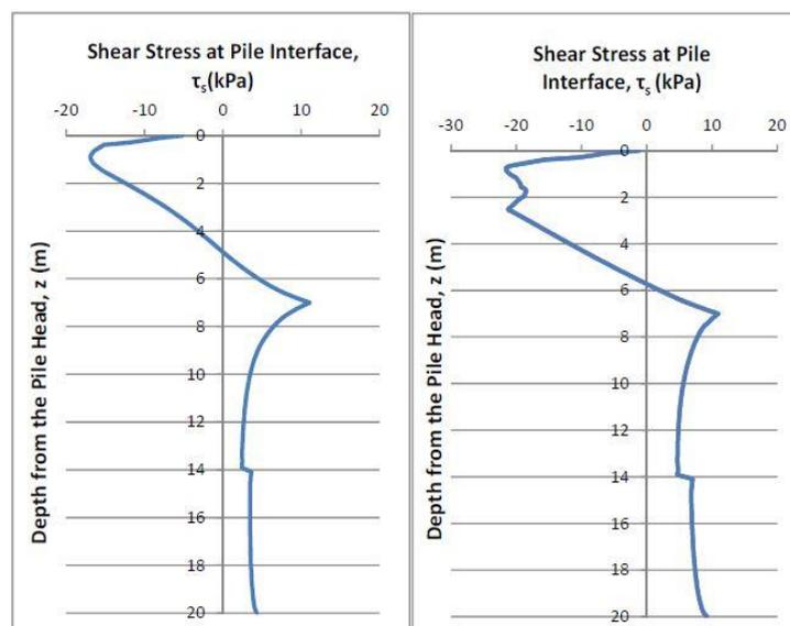
Figure 5: Shear stress distribution, when  $C_p = 5\%$ ; (a)  $h = 3\text{m}$ , and (b)  $h = 7\text{m}$ .
