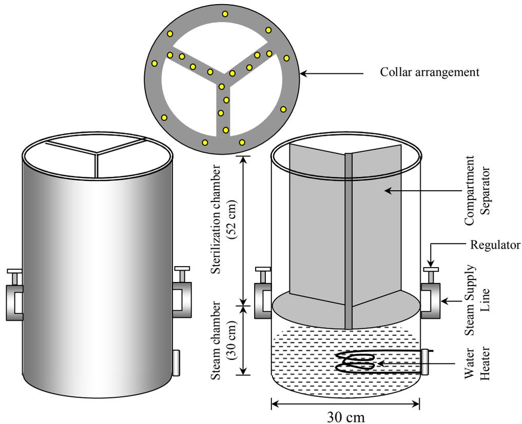
Figure 1: Schematic diagram of continuous operating autoclave
