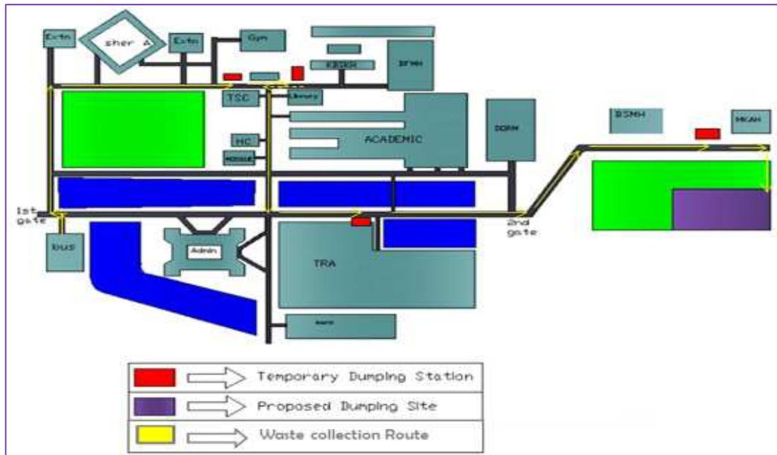
Figure 6: Recommended Layout of waste management system
