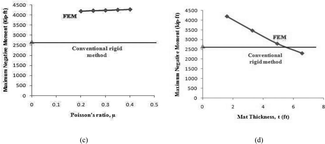
Figure 8: Maximum Negative Moment VS (a) Concrete Elastic Modulus (b) Subgrade Modulus (c) Poisson's Ratio (d) Mat Thickness, in FEM Analysis by SAFE V12
