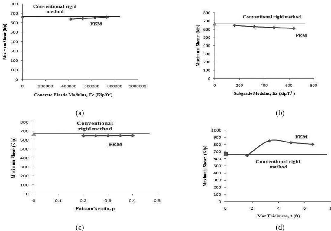
Figure 10: Maximum Shear VS (a) Concrete Elastic Modulus (b) Subgrade Modulus (c) Poisson's Ratio (d) Mat Thickness, in FEM Analysis by SAFE V12
