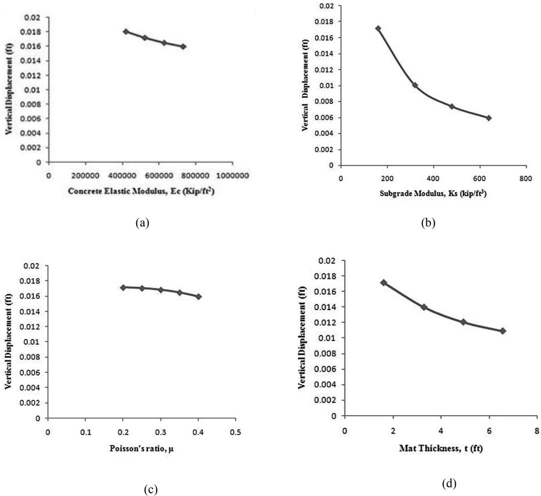
Figure 5: Vertical Displacement VS (a) Concrete Elastic Modulus (b) Subgrade Modulus (c) Poisson's Ratio (d) Mat Thickness, in FEM Analysis by PLAXIS 3D
