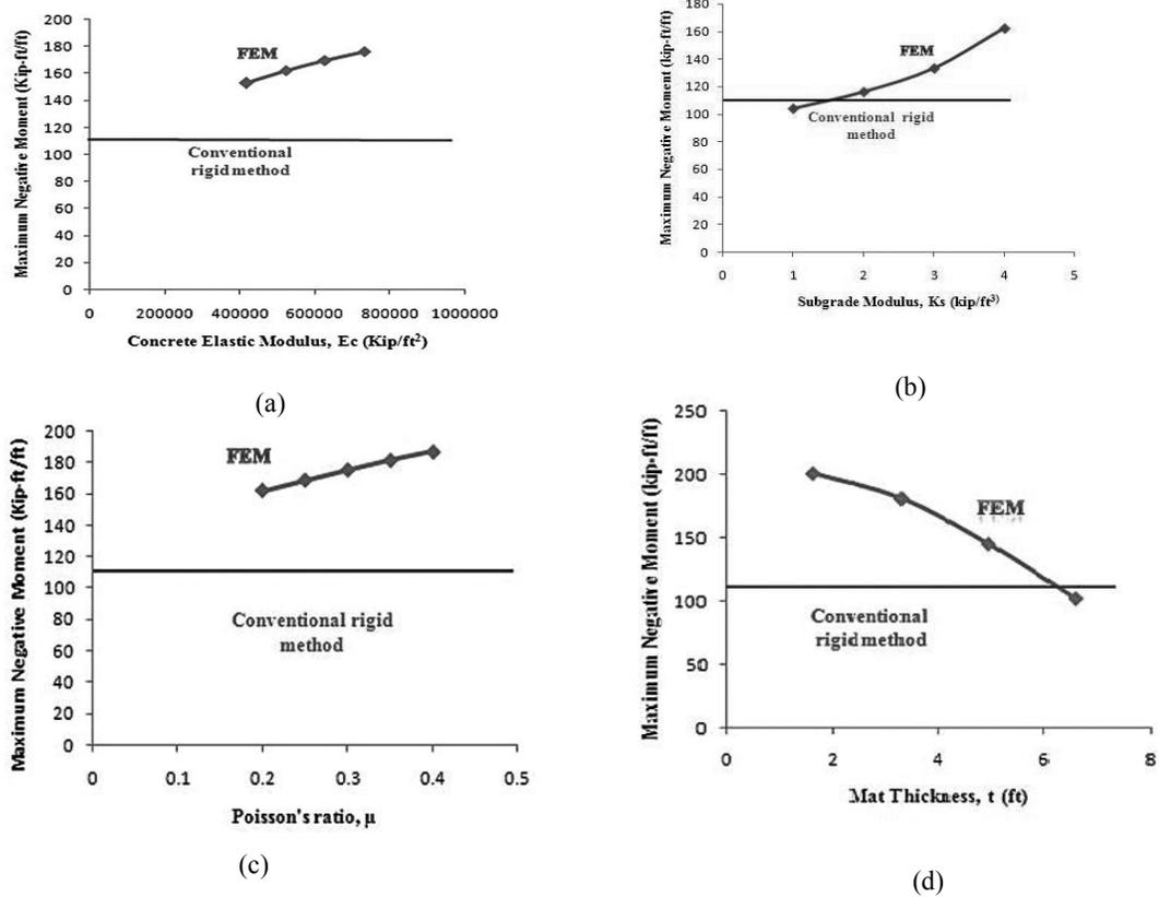
Figure 7: Maximum Negative Moment VS (a) Concrete Elastic Modulus (b) Subgrade Modulus (c) Poisson's Ratio (d) Mat Thickness, in FEM Analysis by PLAXIS 3D
