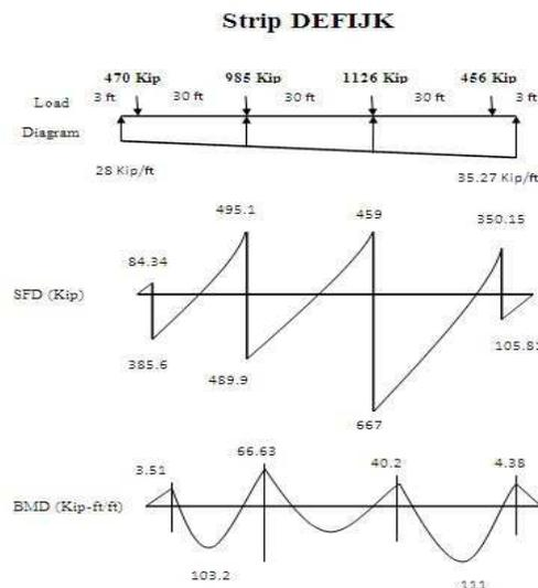
Figure 4: Load, shear force and bending moment diagram of strip DEFIJK
