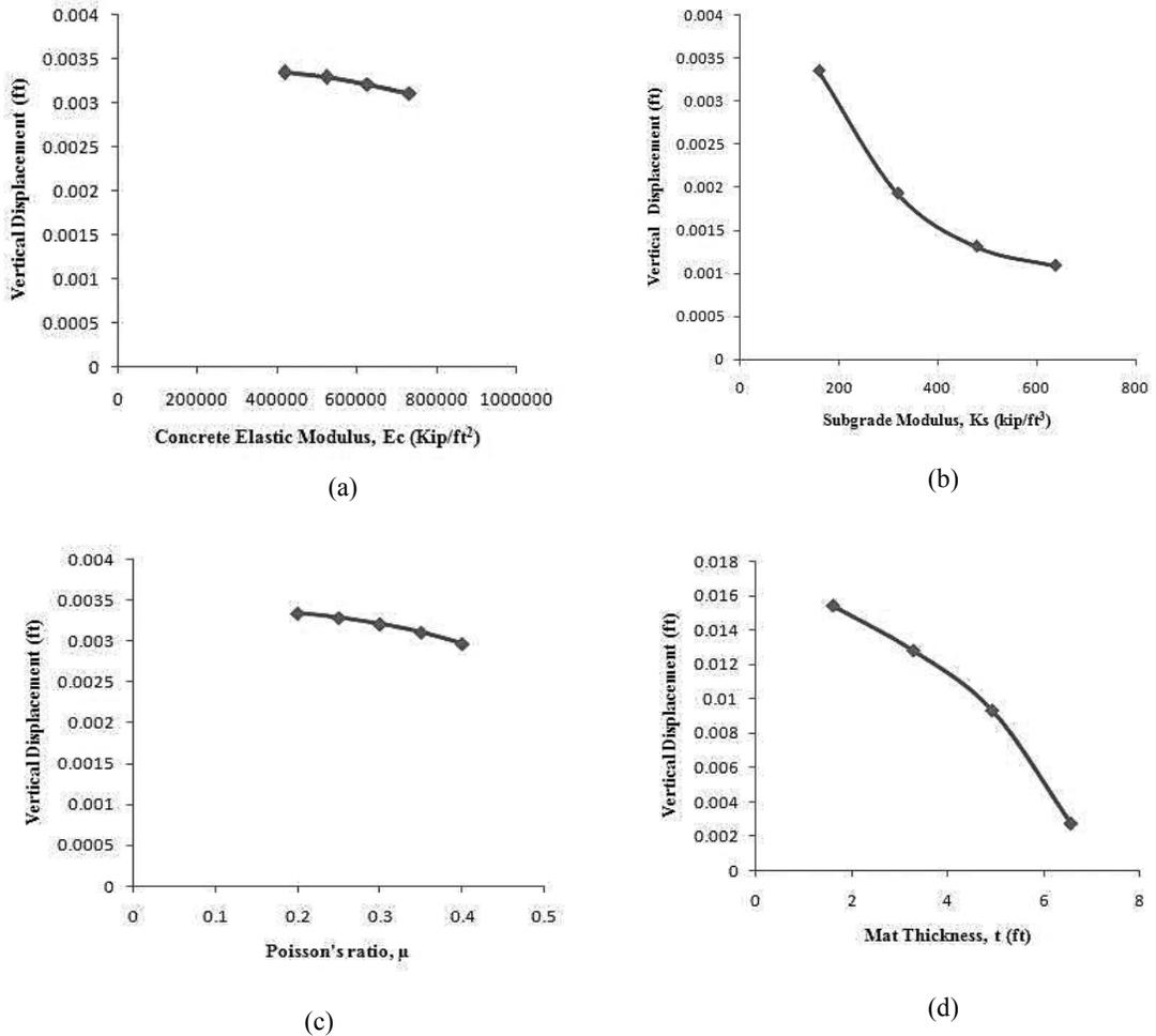
Figure 6: Vertical Displacement VS (a) Concrete Elastic Modulus (b) Subgrade Modulus (c) Poisson's Ratio (d) Mat Thickness, in FEM Analysis by SAFE V12
