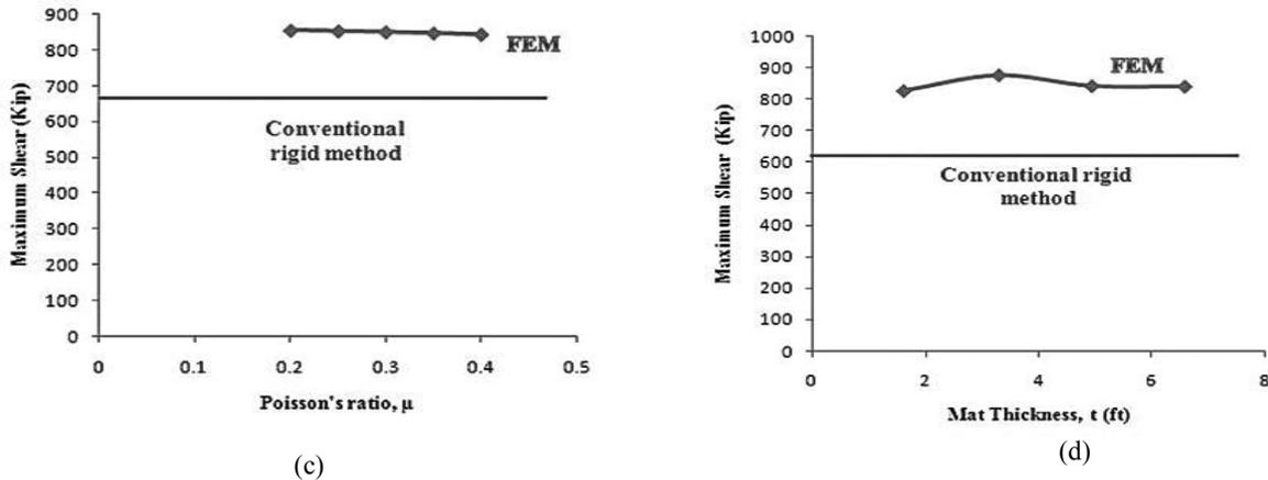
Figure 9: Maximum Shear VS (a) Concrete Elastic Modulus (b) Subgrade Modulus (c) Poisson's Ratio (d) Mat Thickness, in FEM Analysis by PLAXIS 3D
