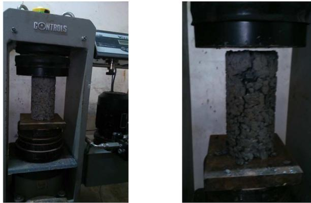
Figure 2: Compressive strength test of no fines concrete
