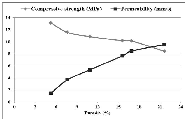
Figure 3.5: Effect of porosity on compressive strength and water permeability
