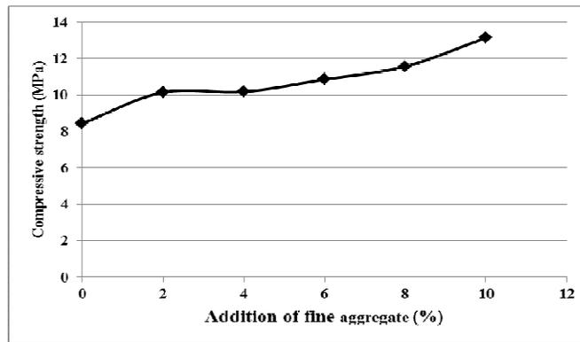
Figure 6: Effect of adding fine aggregate on compressive strength
