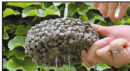
Figure 1: No fines concrete draining water
