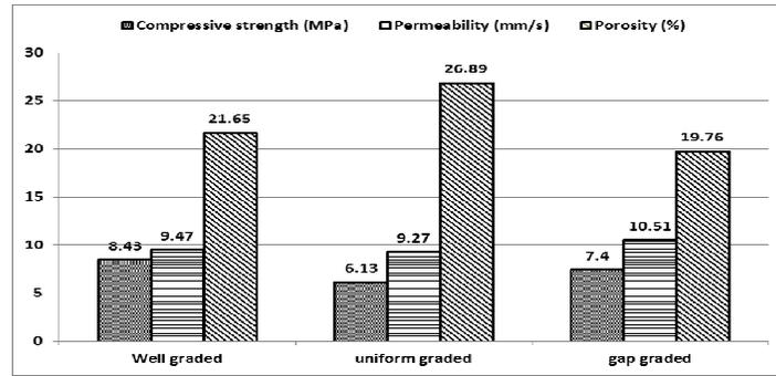
Figure 5: Effect of aggregate gradation on compressive strength, porosity and permeability
