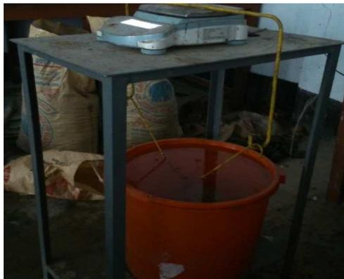
Figure 3: Weight in water of no fines concrete
