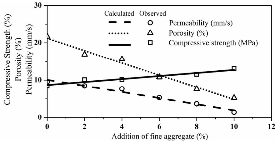
Figure 3.6: Correlation for compressive strength, porosity and water permeability
