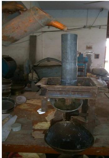
Figure 4: Constant head water permeability test
