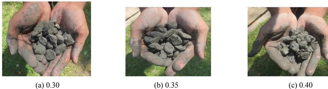
Figure 2: Determination of water/cement ratio
