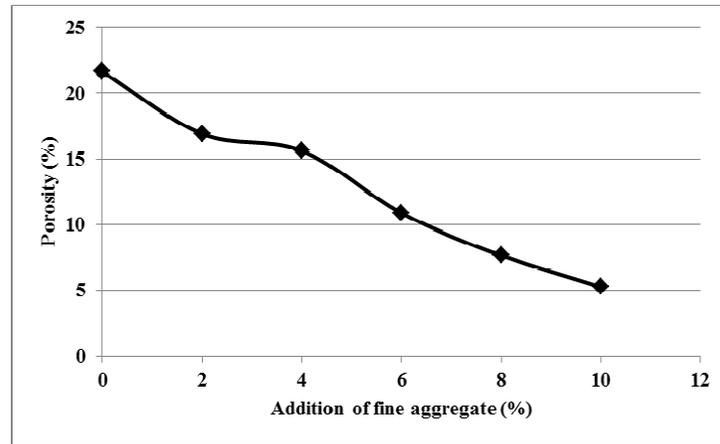
Figure 8: Effect of adding fine aggregate on porosity
