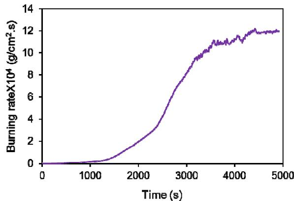
Figure 2: The rate of burning rate of the PMMA slab at a radiation rate of 12.55 kW/m<sup>2</sup>.
