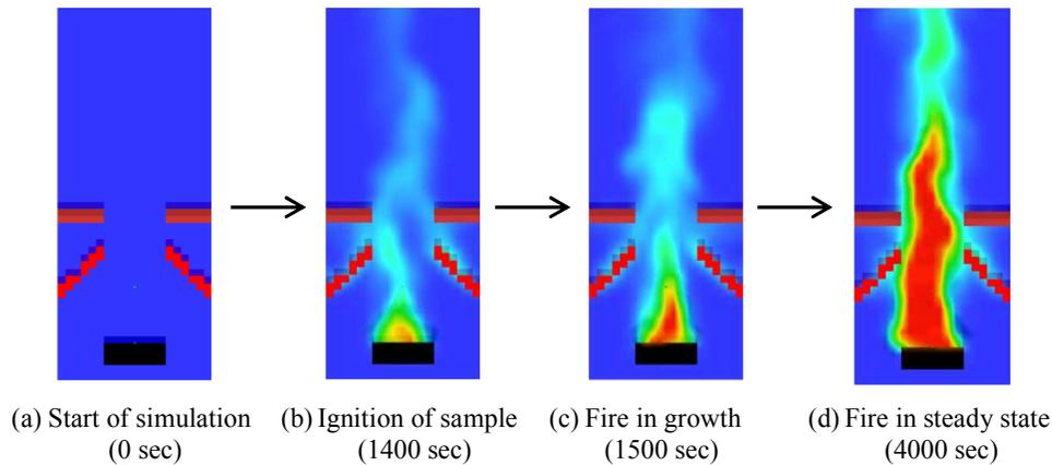
Figure 4: Burning of fire at different stages produced by the PMMA slab.
