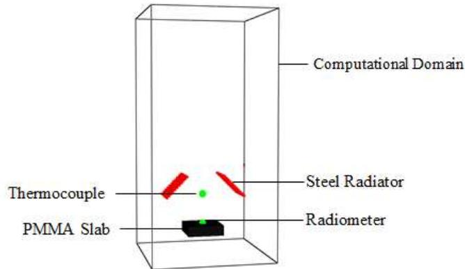
Figure 1: Set-up of the computational domain for the simulations of fires produced by a PMMA slab.
