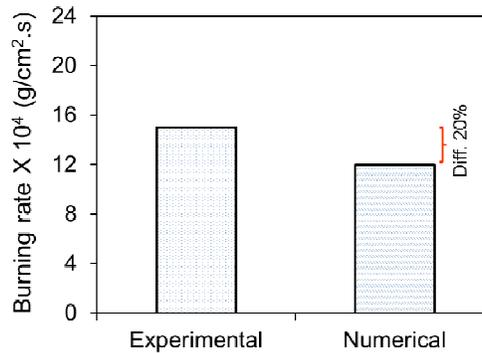
Figure 3: Comparison between the experimental and numerical steady state burning rates of PMMA slab.
