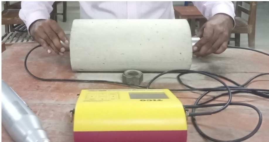
Figure 3: Ultrasonic Pulse Velocity (UPV) test performed over cylinder
