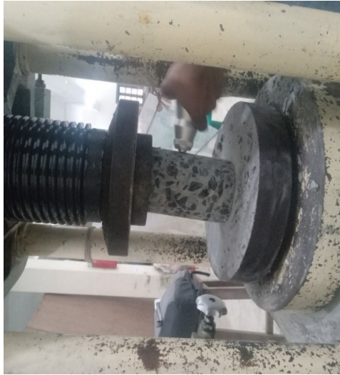
Figure 2: Rebound Hammer (RH) test performed over core cylinder
