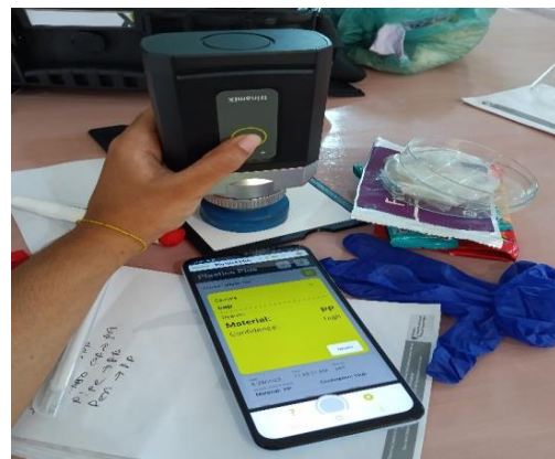
Figure 6: Plastic Fraction Identification by NIR Spectroscopy
