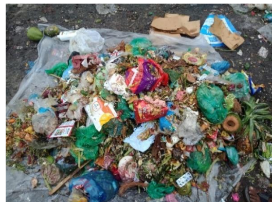
Figure 2: Mixed SW from a van was collected on a sheet and then the weight of the total SW was found
