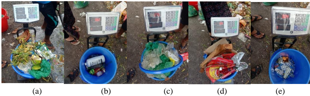
Figure 3:Composition of waste (a) Biodegradable Waste (b) Plastic Bottle (c) Polythene and Plastic Sheet (d) Paper (e) Medical Waste
