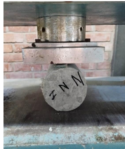
Figure 2: Splitting tensile strength test
