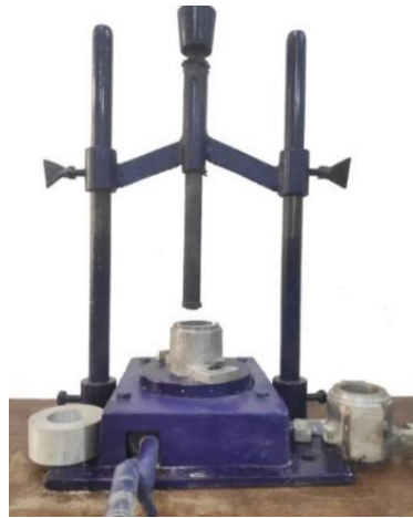
Figure 1: Compaction hammer with loading frame and compaction mould.
