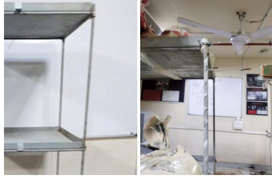
Figure 6: Column jacketing with rubber
