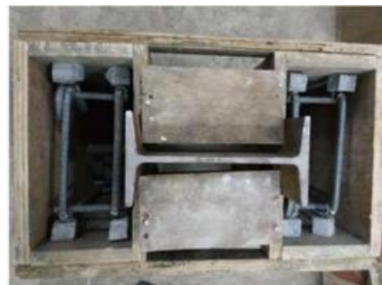
Figure. 2(b): Shuttering of specimen
