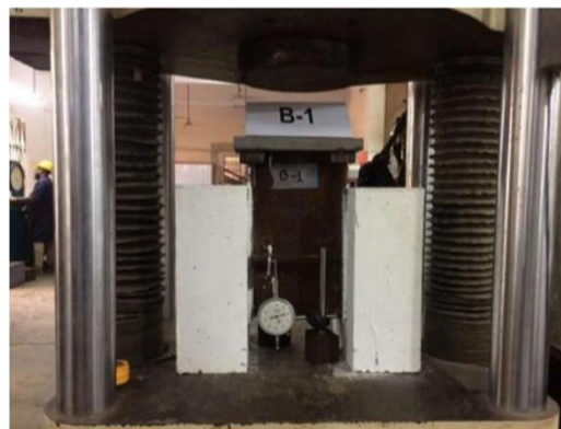
Figure. 4: Test setup and instrumentation(Kabir & Begum, n.d.)
