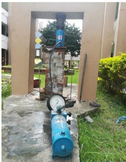
Figure 2: Experimental setup for the compressive test of column
