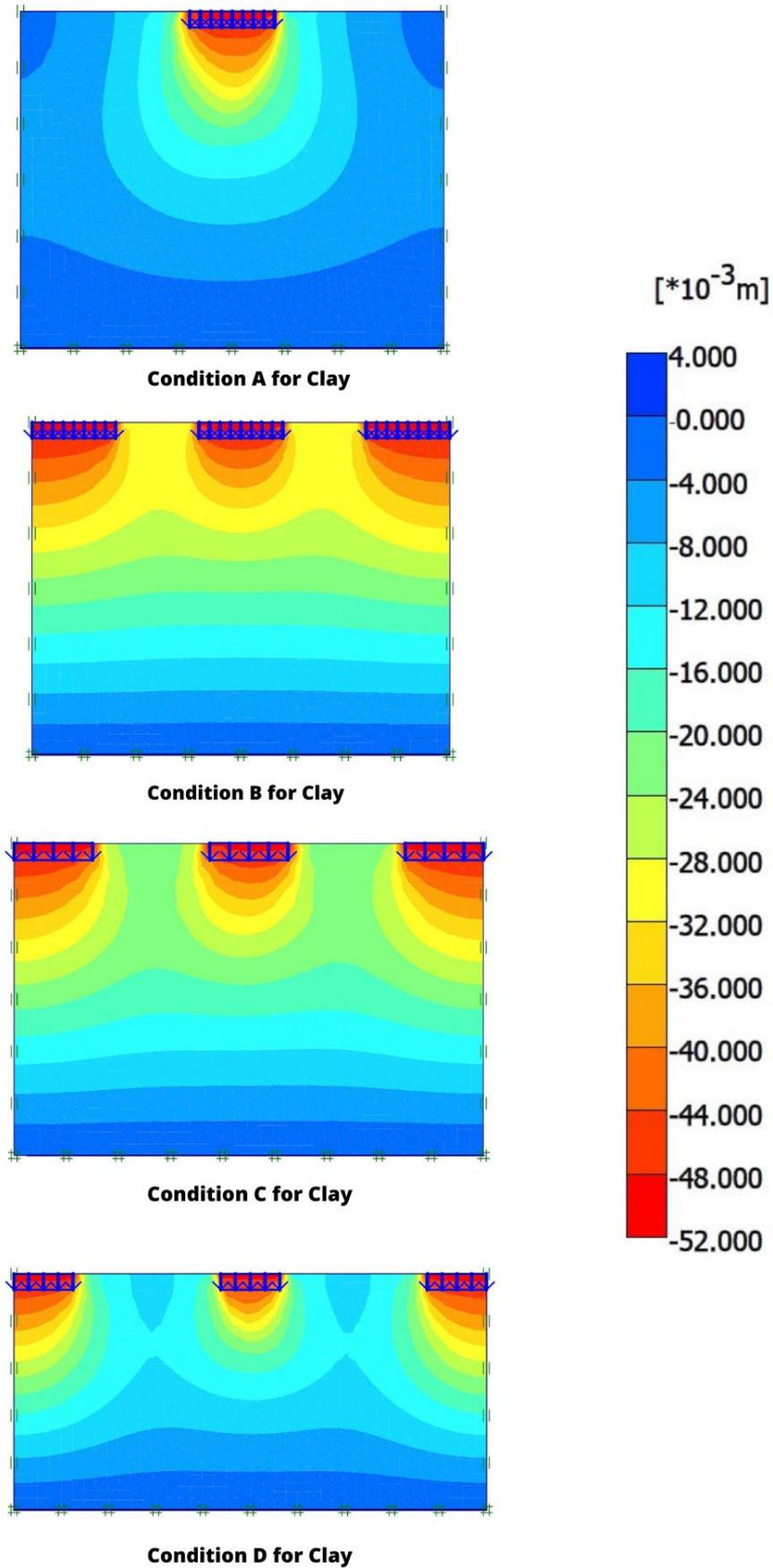
Figure 7: Conditions on Clayey Sand from PLAXIS (condition A, B, C, D)
