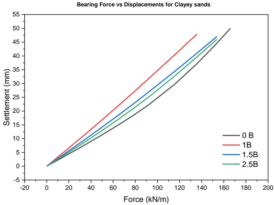
Figure 8: Graph on Bearing Force vs Displacements for Clayey Sand
