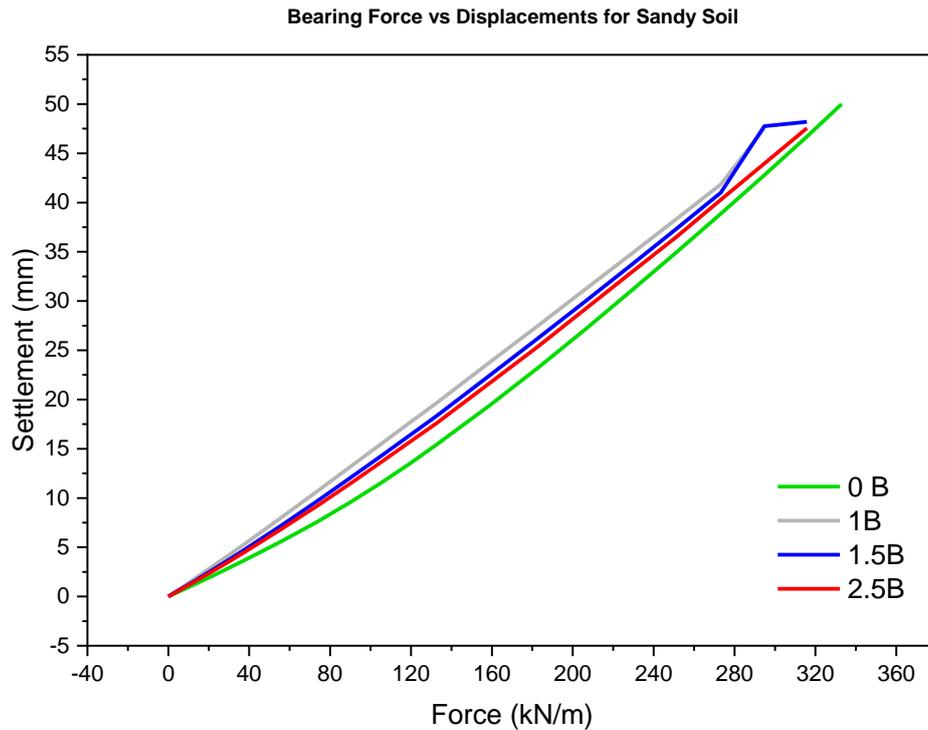
Figure 6: Graph on Bearing Force vs Displacements for Sandy Soil
