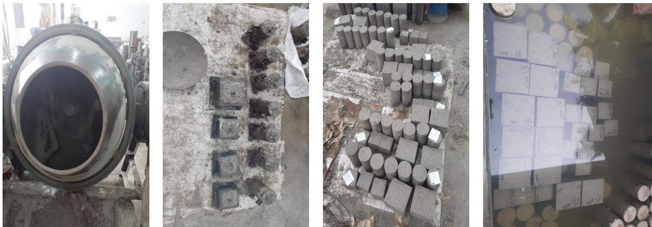
Figure 3: Mixing, casting and curing of concrete
