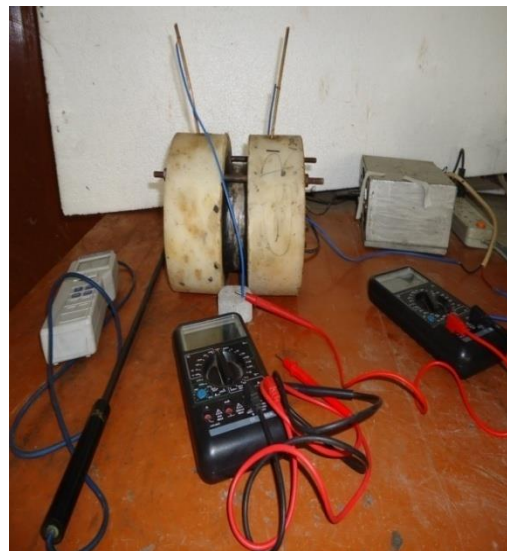
Figure 3: RCPT test setup; (a) Schematic diagram and (b) Image of the test set-up
