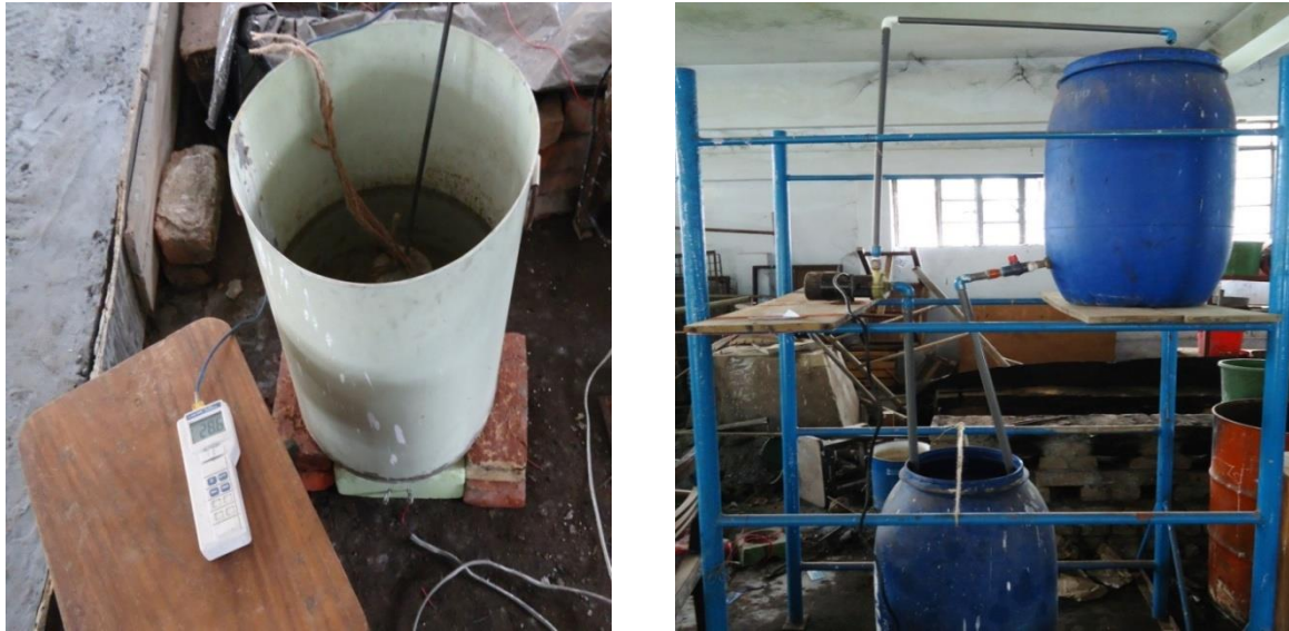
Figure-4: Thermal diffusivity test (a) Boiling Phase and (b) Cooling Phase
