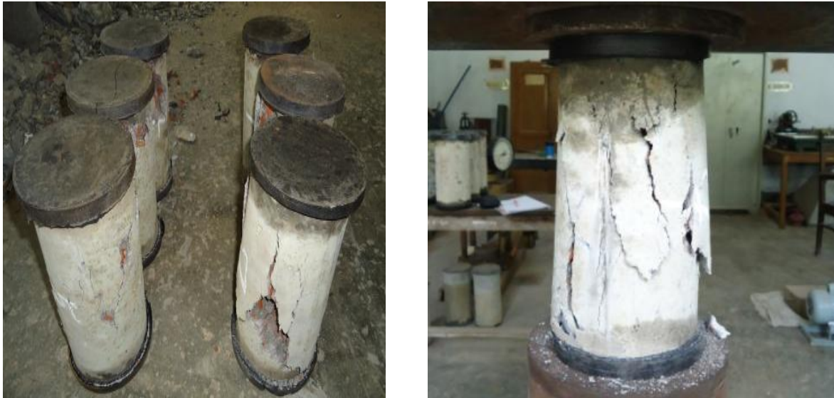
Figure 2: (a) Compression strength test of specimen, (b) Fracture pattern of one of the samples
