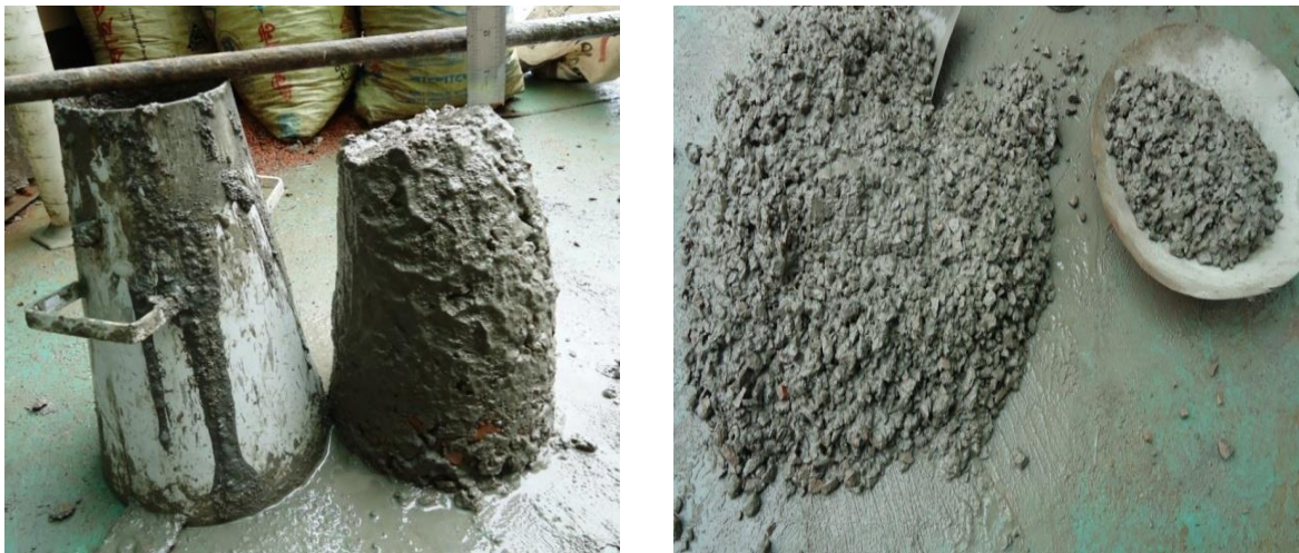
Figure 1: Concrete mix and measurement of slump value
