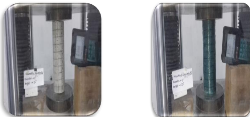
Figure 2: Wrapped and Unwrapped specimens under static loading
