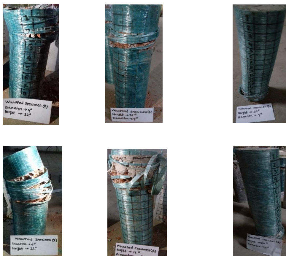
Figure 9: Failure pattern of wrapped cylindrical specimens.
