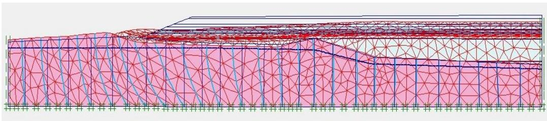
Figure 3: Deformed mesh generated using sand drain
